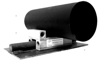
When round bar has been welded to an I-beam, Bar Hoppers allow APP ProTek Wear Pads to be used without removing the round bar. Our composite material bar hoppers are installed over the round bar so that the pipe rests on the top plate of the bar hopper. This design eliminates round bar point loading.
