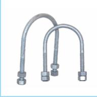
**Standard U-bolts:** Standard U-bolts usually are made of carbon steel or variations of stainless steel. There are also finishes and coatings that can improve their durability, such as zinc plating, fluoropolymer coatings, or hot-dip galvanization.
