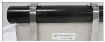
Run a final silicone bead around the upper edge of the pipe shoe.
