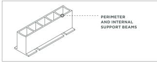
② Run a continuous silicone bead around the perimeter of the ProTek Pipe Shoe and along the internal support beams.
