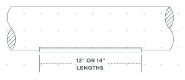
ProTek Composite Wear Pads are designed to prevent metal-to-metal contact in piping systems. They effectively isolate the pipe from contact with I-Beams, guides or concrete supports. These areas are the most susceptible to corrosion and cost millions to repair and maintain. Our wear pads are the most cost-effective solution to piping system corrosion.
