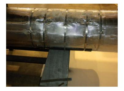
**Test Procedure:** Load of 3,000 pounds was applied to the cradle. The test apparatus was moved longitudinally across the I-beam (4 inches in each direction). This was to simulate thermal cycling over 20 years of operation, with a safety factor of 4.
