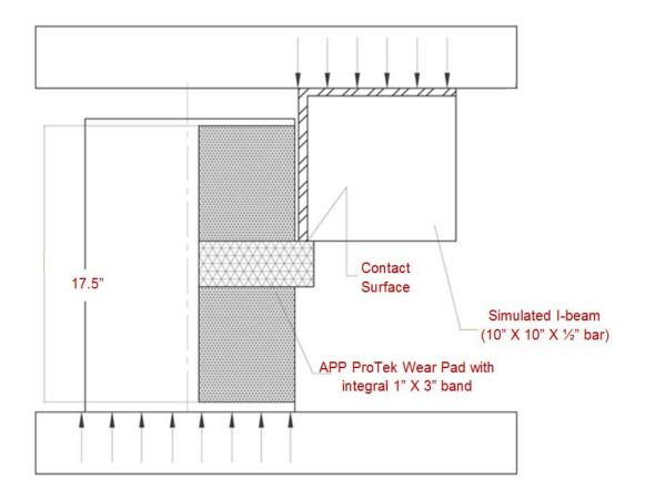
**Test Results:** The epoxy was found to be able to handle overlap shear loads in excess of 44,000 pounds. The test was ended at a load of 44,437 pounds because the raised ring had been point loaded and had begun to crack, but even at this high load, there was no epoxy failure or separation of the pipe from the wear pad.
