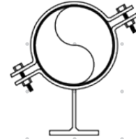
FIGURE 3020 Fabricated with two clamps to hold the pipe in place.
