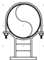
FIGURE 3210 Fabricated with two cradles and comes with two u-bolts to hold the pipe in place.
