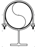
FIGURE 3010 Fabricated with two cradles and comes with two u-bolts to hold the pipe in place.
