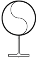
FIGURE 3000 A standard T-Slide Metallic Pipe Shoe and is welded onto the pipe.
