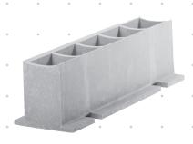
ProTek Composite Pipe Shoe is a UV-resistant, non-metallic solution for elevated or insulated piping systems at the support points. It has 150,000 lbs. of compressive strength, a temperature range of -320°F to +400°F and is resistant to chemical attack. It is the optimal support for insulated or elevated piping systems in plants or refineries, both onshore and offshore.
